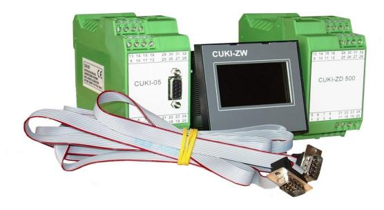
Leakage central-blocking device type CUKI -05 is designed for controlling the earth resistance of a grid (including frequency converters) for rated three-phase voltage of 500V/50Hz with isolated star point on the transformer (system IT), to be used with equipment designed for working on the ground and in underground mining in mine face pits in non-explosive conditions, in conditions without methane explosion hazard and classified as A coal-dust explosion hazard.
